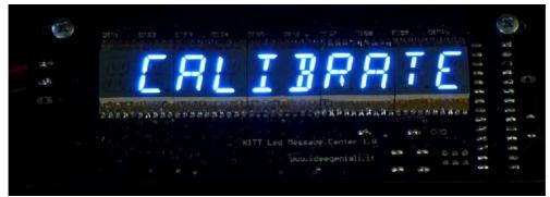
Display dimensions: 13x96mm; Board dimensions: 53x134mm
